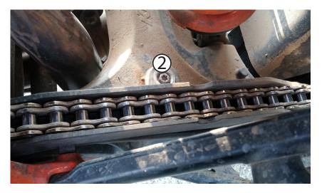
② Use T30 torx to remove this screw that holds chain guide in place. On top of swingarm, inboard of chain in location shown. Leave washer in place.
