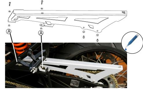
Place aluminum spacers into OE metal cup washer at two front locations as shown(A). Use thread locker on all screws. Insert M5 allen screws with washers and gently tighten. Insert M6 Torx screws with washers at rear mount points and tighten.
