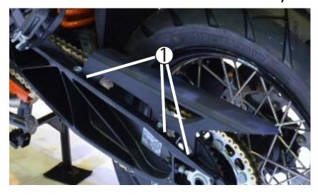
Use T30 Torx to remove three (3) fasteners holding OE plastic chain guard in place. Remove guard.
